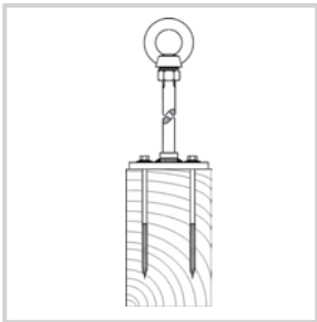
Screwed into wooden rafters (no base plate, with four screws)
